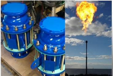
The Paradox Deflagration Flame Arrestor, is designed to stop the propagation of a degflagration beyond the capabilities of a conventional end of line flame arrester. They are ideal for **short flare** stacks (<60ft.) with a ninety degree elbow at the bottom. The deflagration arrester is bidirectional and will stop both low and high pressure deflagrations.
