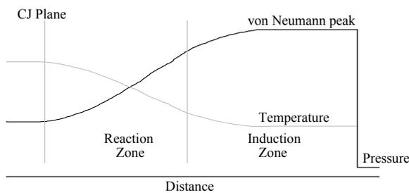
The region between the shock front and the start of energy release is called the von Neumann spike. The gas pressure etc. in this region are given by the non-reactive shock relationships. In this region the initial reactants dissociate with a finite induction period before
