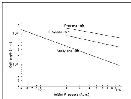
A strong relationship can be observed between the chemistry and cell size in gaseous detonations. The cell size is a convenient parameter determined from the average width to length of the roughly diamond pattern left on a sooted surface. The cell width is also a measure of the average spacing of the transverse waves across a detonation front and the average time between collisions. It is also possible to demonstrate a link between an average induction zone length and cell size.
