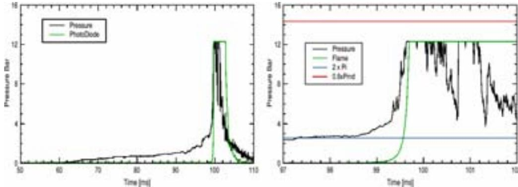
**Figure 6.2** The rapid flame acceleration occurring when flame arrives during deflagration test on an overdriven detonation flame arrester
