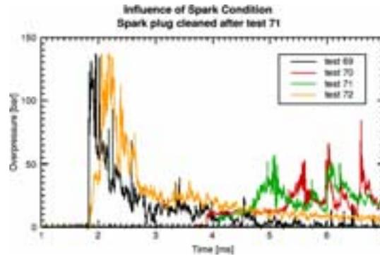
**Figure 6.3.3** Influence of spark energy on flame acceleration
