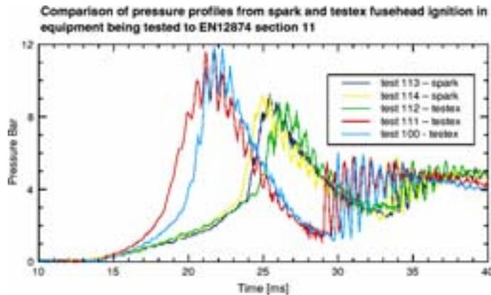
**Figure 6.3.2** Comparison of ignitions in 43% hydrogen air mixtures with testex fuseheads and high energy spark
