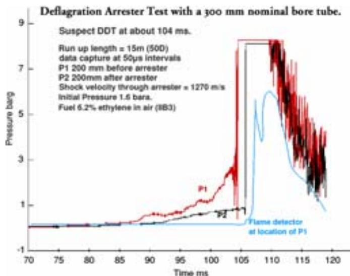
**Figure 6.1** Transition to detonation within 50 pipe diameters in a 300 mm nominal bore pipe. Initial pressure 1.6 bar, temp 10°C. The data capture system was set for deflagrations and hence it is impossible to establish exactly what is occurring in the transition region
