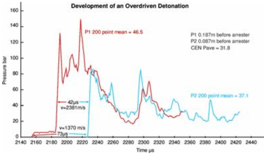
**Figure 6.6.1** Pressure Histories of from two sensors located 100 mm apart. Tests from a 50mm nominal bore tube. The transient nature of an overdriven detonation is clearly shown
