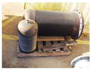
temperature could rise sufficiently to initiate a potentially destructive explosion. To prevent such a sequence of events flame arresters have been installed, in systems, immediately upstream and downstream from the catalyst bed to stop and quench the flames resulting from any unexpected ignition. The major problems encountered when attempting to design flame ar-
