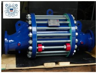
*The Paradox Detonation Flame Arrestor*, represents the best technology for value in flame arrestor protection. They prevent flame propagation by absorbing heat and dissipating supersonic pressure waves, using multiple spiral wound crimped ribbon flame cells staged with turbulent creating screen sections.
