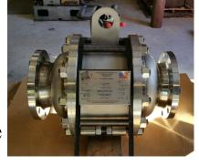
The arrestor provides the option of removal of the flame cell (element) for easy cleaning and replacement without disconnection of the pipe connection flanges. Standard housing construction is carbon steel and stainless steel. The element is available in 304 SS, 316 SS & Hastelloy. Special material and protective coatings are available on request, except for Aluminum. We do not fabricate any aluminum flame arrester products and consider them to be a liability.
