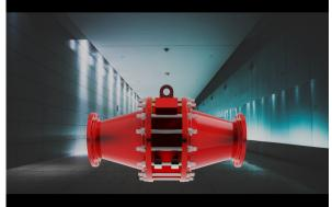
The Paradox Standard In-Line Flame Arrestor prevents flame propagation by acting as a heat sink, cooling the flame front to cause it to be extinguished. This heat sink is made from spiral wound crimped ribbon that
