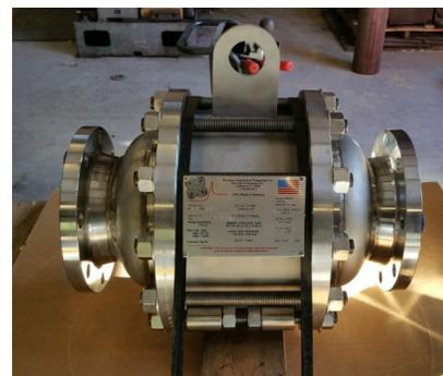
The arrestor provides the option of removal of the flame cell (element) for easy cleaning and replacement without disconnection of the pipe connection flanges. Standard housing construction is carbon steel and stainless steel. The element is available in 304 SS, 316 SS & Hastelloy. Special material and protective coatings are available on request, except for Aluminum. We do not fabricate any aluminum flame arrestor products and consider them to be a liability.
