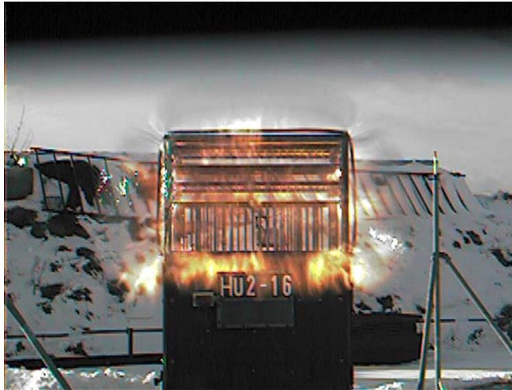
Figure 4 Example of hydrogen explosion experiment 28 ms after ignition.
