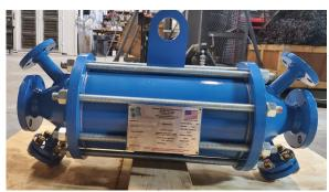
of 0.70 is classed by NEC as Group "B". Previously detonation flame arresters approved by the USCG for **Propylene Oxide** were mistakenly Group C, (gases having an MESG greater than 0.65mm). The problem being not all gases react the same when ignited within their prospective explosion limits, refusing to react in the same manner as similar gases that have been classified by using the **MESG as the criteria**.
