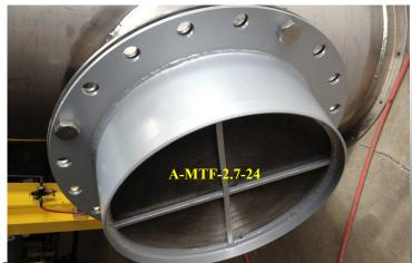
The Paradox MTF Flame Arrestor, prevents flame propagation by acting as a heat sink, cooling the flame front to cause it to be extinguished. This heat sink is made from spiral wound crimped ribbon that allows gas to flow with a minimum pressure drop.
