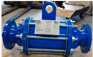
The Paradox Deflagration Flame Arrestor, is designed to stop the propagation of a deflagration beyond the capabilities of a conventional end of line flame arrester. They are ideal for **short flare stacks** (<60ft.) with a ninety degree elbow at the bottom. The deflagration arrester is bidirectional and will stop both low and high pressure deflagrations.
