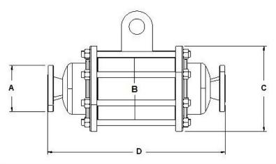
Detonation Flame arrester Specifications
