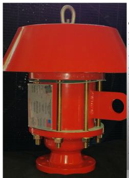
The Paradox End of Line Flame Arrestors, are designed for free venting while simultaneously preventing flame propagation of confined and unconfined low pressure deflagrations. They prevent an ignited atmospheric vapor cloud from propagating beyond the Flame Arrestor into the line or tank.
