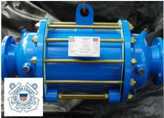
The Paradox Detonation Flame Arrestor, represents the best technology for value in flame arrestor protection. They prevent flame propagation by absorbing heat and dissipating supersonic pressure waves, using multiple spiral wound crimped ribbon flame cells staged with turbulent creating screen sections.
