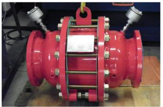
The Paradox In-Line Flame Arrestor, prevents flame propagation by acting as a heat sink, cooling the flame front to cause it to be extinguished. This heat sink is made from spiral wound crimped ribbon that allows gas to flow with a minimum pressure drop.
