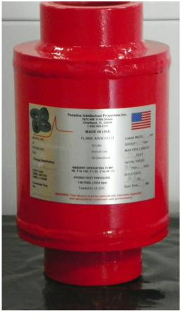
Standard housing construction is carbon steel with 3000# threaded half coupling connections (NPTF). Stainless steel and other alloys are available upon request. The standard element is 304SS and 316SS or hastelloy is also available.
